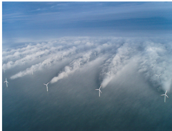
Figure 1: Turbulent airflow from wakes is exposed due to extreme humidity in the air. Picture by Christian Steiness (12.02.2008) [13]
