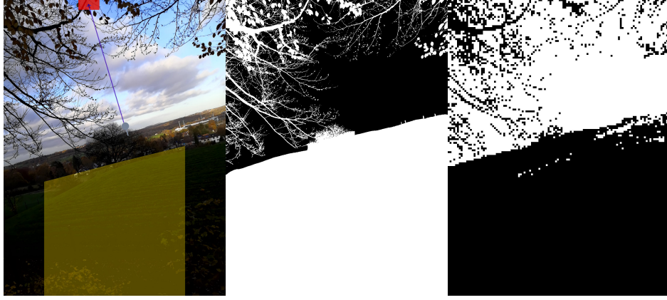
Figure 19: Left image: the sky region (red) is selected by following the direction of the wind turbine direction, and the ground region (yellow) is selected using the DEM depth data. Middle image: ground truth map with white marking foreground pixels and black marking background pixels. Right image: output of the sky segmentation algorithm, white marking sky pixels and black marking non-sky pixels.
