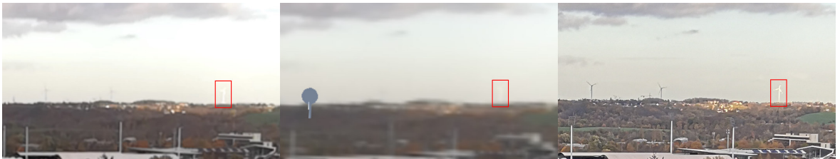
Figure 36: Left: Camera image acquired using the AR Foundation Camera Manager with the highest possible resolution. Middle: Image rendered on the screen inside the Unity AR Application. Right: Camera image taken by smartphone. The red-marked real-world wind turbine is around 7.24km away.
