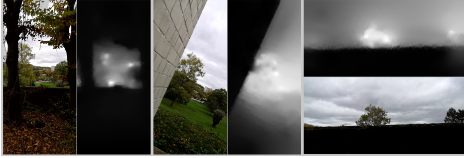
Figure 23: Purposive sample representing the Informatikzentrum Sequence with corresponding SfM depth maps. Dark colors represent close-depth, and bright colors represent far-depth estimations. For the entire scenes, see Figure 41 in Appendix.
