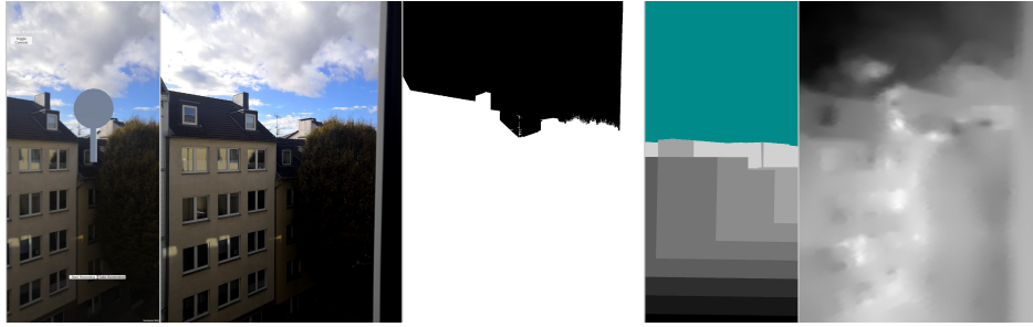
Figure 20: Example visualization of a scene. From left to right: screen image, camera image, ground truth map (white representing foreground and black background pixel), DEM depth map, SfM depth map. Depth maps: brighter color equals greater distance; cyan marking regions with no depth.
