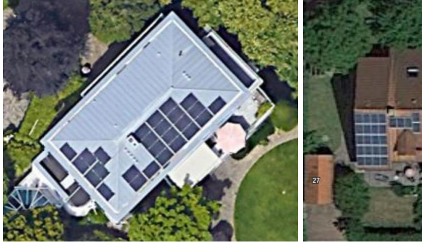
Figure 5: Left is the first case study object consisting of roof with 4 segments low slope angle and a few, small chimney obstacles. Right is the second case study object. A semi-detached house with two roof segments, a dormer, chimney and a large window. Both houses are shown being oriented such that north is up. (Source: GoogleEarth)
